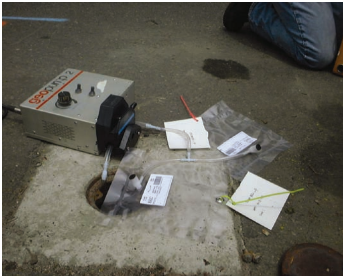
Figure 10. Photograph of peristaltic pump and one-liter Tedlar bags (replicate sample) used for sampling dedicated vapor probes.
