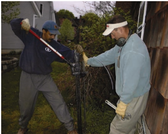
Figure 21. Retraction of Retractable Tip prior to sampling.
