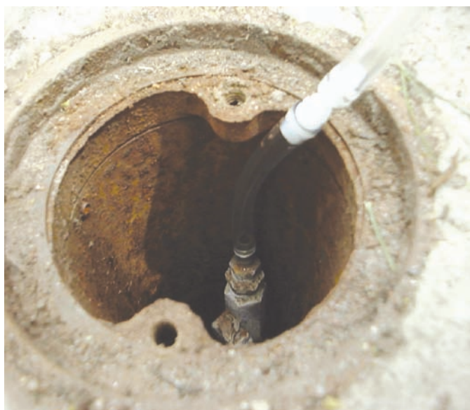
Figure 8. Photograph of valve used to seal dedicated probes, PVC barbed fitting, and Teflon ® tubing used for sampling.
