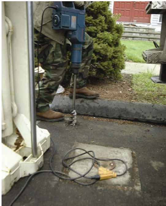
Figure 17. Creation of hole in asphalt prior sampling with GVP kit.
