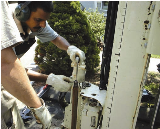
Figure 15. Photograph of metal rod used to push out the expendable point.
